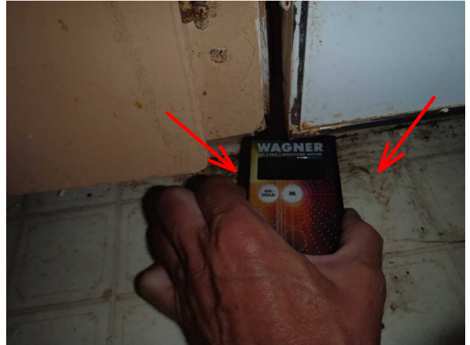
base area of dishwasher is noted with high moisture readings....expect floor damage here...
