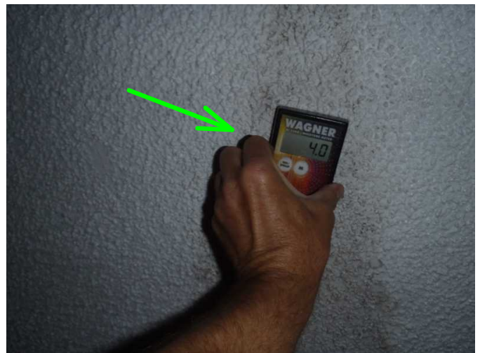
staining at ceiling area is noted low moisture...appears was past issue...
