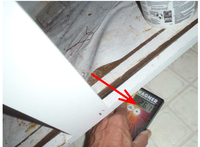
cabinet area floor is noted high in moisture..expect damage to under layment...
