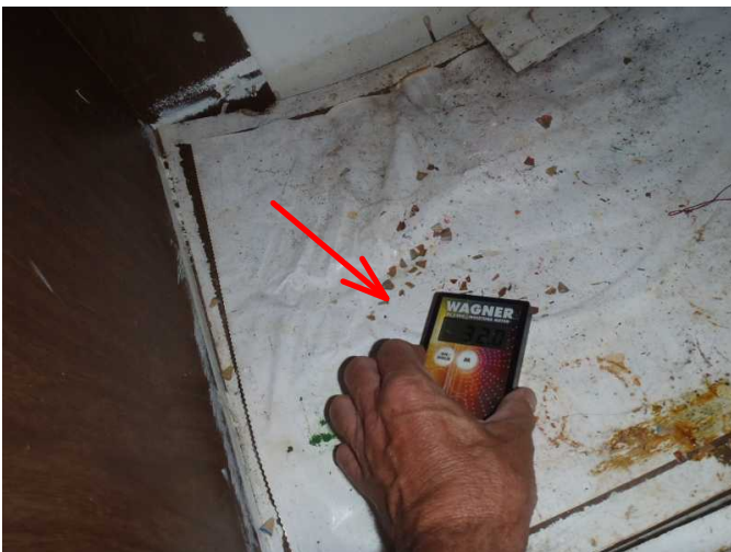
floor of cabinet is also noted high in moisture...expect floor under cabinet to be damaged..
