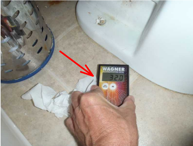
floor at toilet in main bath at 11900 is noted saturated again...as is in master...
