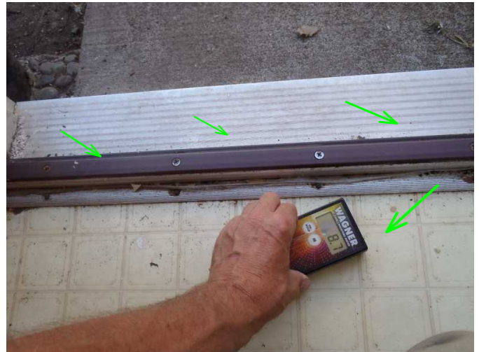
threshold appears solid and floor area at back door is noted low in moisture...
