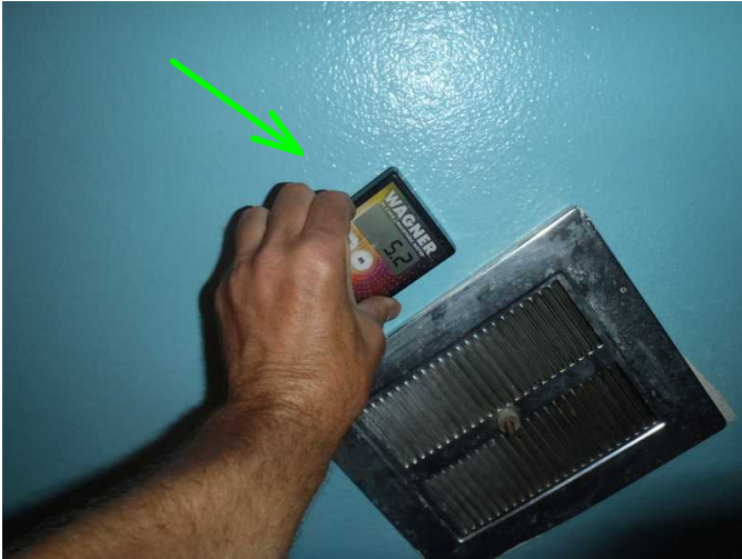
ceiling fan is noted operable...and low moisture at ceiling area...
