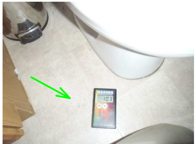
toilet is noted solid to floor and operable...floor is noted low in moisture at rest of areas...
