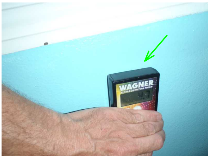
low moisture is noted at all areas of exterior wall ...
