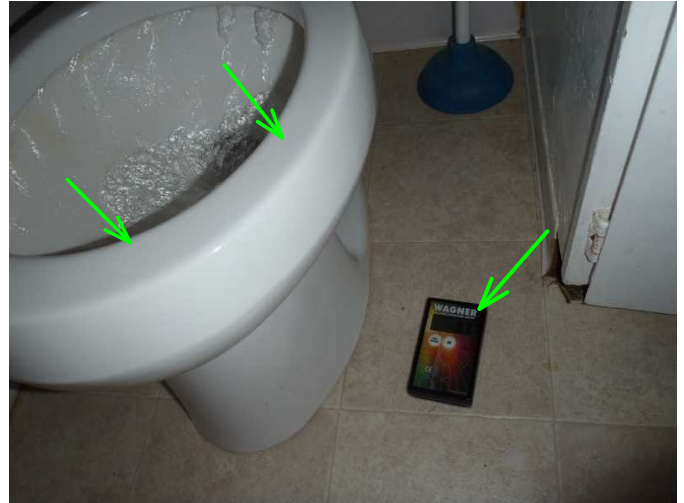
toilet is noted operable...and floor moisture is noted low...
