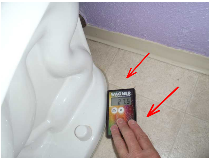
one area of master bath is noted with high moisture at floor...back corner of floor at right side...
