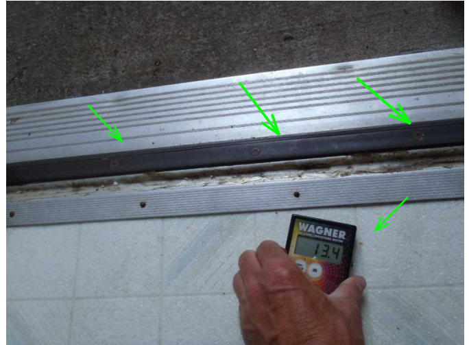
threshold is noted solid...moisture at floor is noted low...good..
