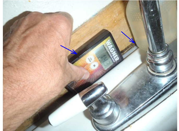
low moisture is noted at wood back splash...is stained...not mold...
