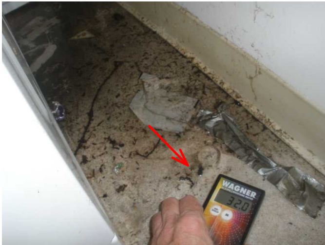
and noted standing water behind washer are...and noted saturated moisture meter reading...
