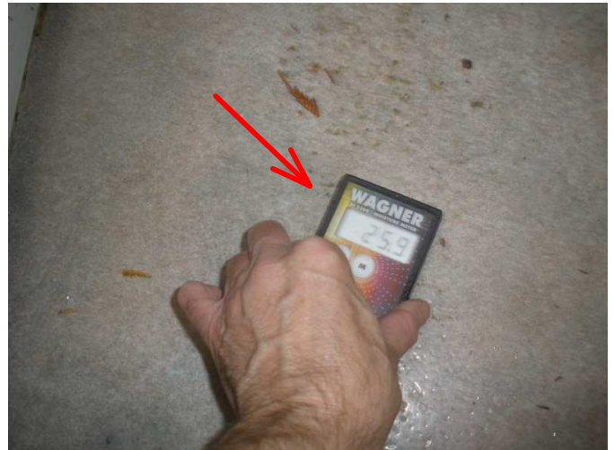
high moisture is noted here at floor by dryer...
