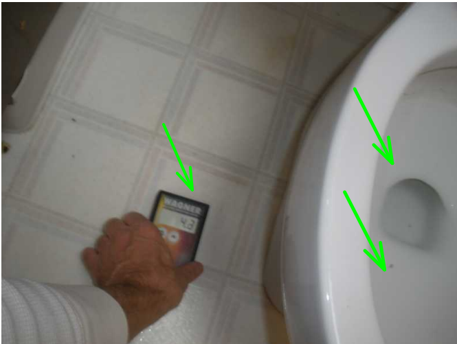
toilet is noted solid to floor and moisture is noted low...toilet was shut off at feed and turned on and tested...
