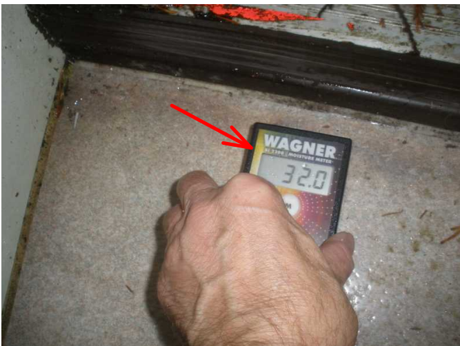
this is reading that means is saturated..is highest moisture meter can read...damage is noted here...
