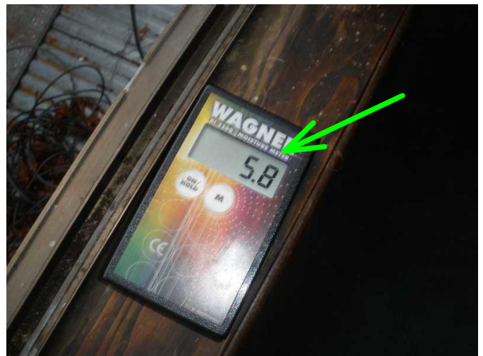
low moisture noted at window sills...
