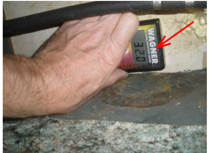
noted black mold at lower walls under cabinets...and moisture reading of 32 %
