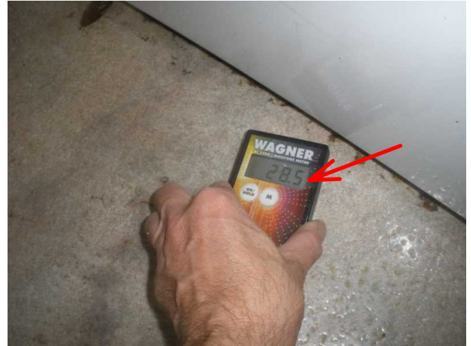
and at front of dryer area...moisture meter can read up to 4 inches into floors and walls...
