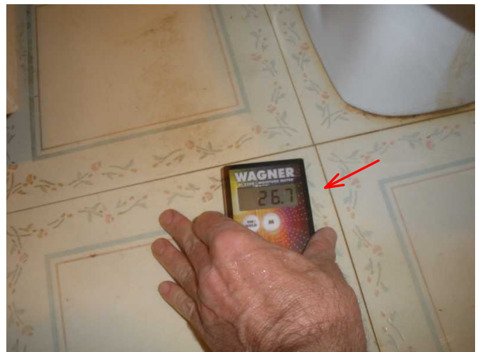
high moisture is noted at toilet area of floor as well..appears to flow from tub area...
