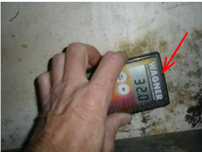
noted more black mold and moisture reading at 32% at lower drywall walls of kitchen area...
