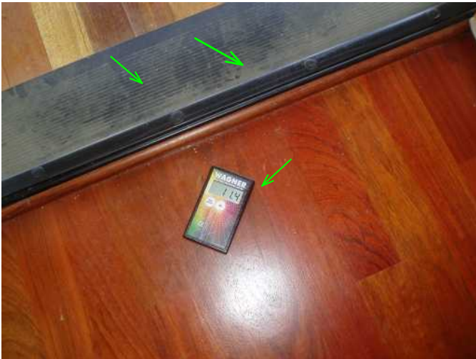
threshold and weather stripping around door are noted fine..no high moisture at floor noted at entry door..
