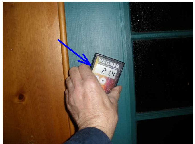
high mositure noted at window trim in dining area...is noted that the exterior is not sealed well...
