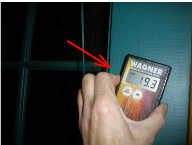
all throughout home is noted with higher moisture content of exterior wood trim...is due to no heat and damp areas..
