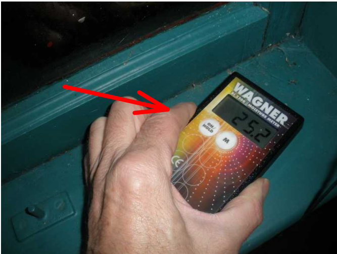
high moisture noted at exterior window sills at main level of home...appears to be too damp...leave heat on...
