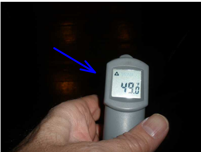
temperature of floor of home...is very cold...no insulation noted at under floor crawl area...
