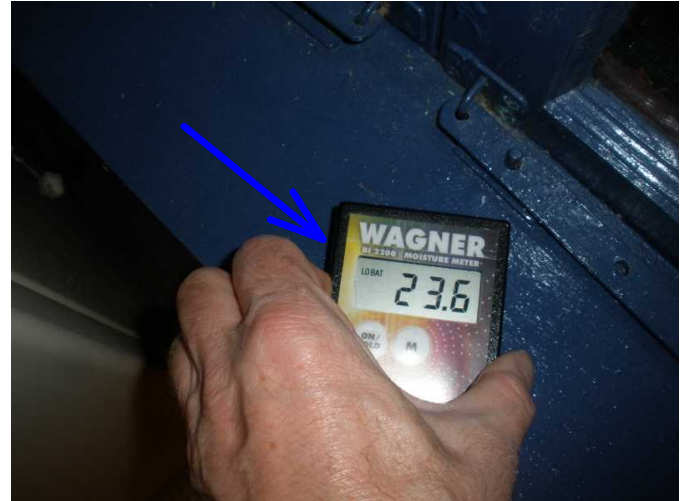
first floor bath window sill is noted to high...should not be above 20 % and the whole home is very damp....
