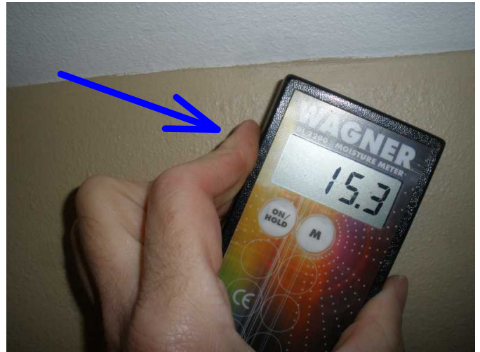
am noting wall to bed 2 ceiling is fine...but is higher than normal...home has no heat on and can get damp...
