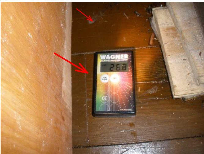
noted high moisture at floor area by wood stove..appears is coming from wall of sink area...
