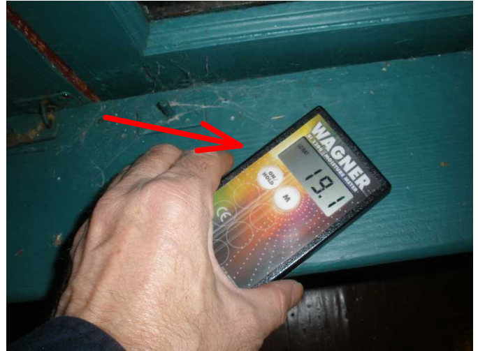
high moisture noted at window sills in study area...
