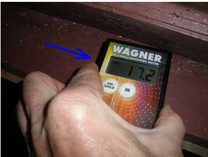
higher moisture noted at window areas...at sills...noted at all exterior wall sills...run all heaters to keep home dry...
