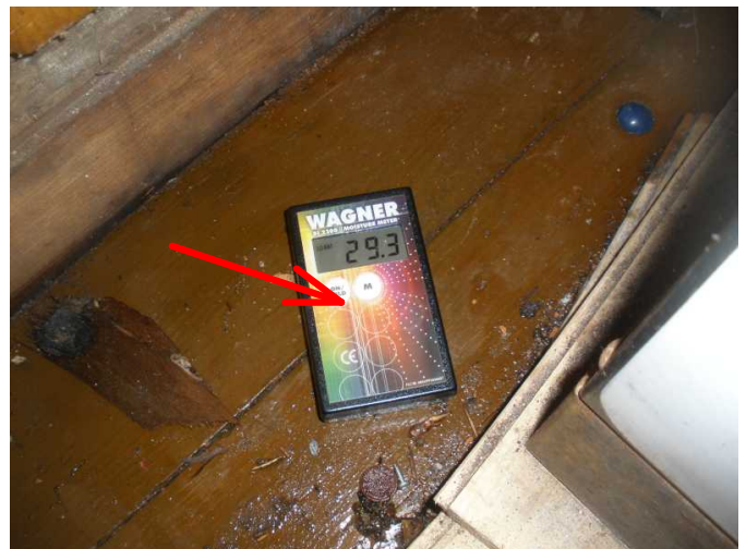
high moisture readings noted here at wood stove area behind wood stove in kitchen....
