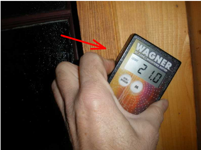
higher moisture noted at trim at study area windows...appears all exterior wall areas have higher moisture...
