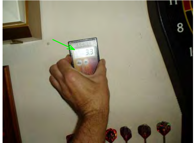
again, at random, checked for moisture in exterior walls and all is fine...good...
