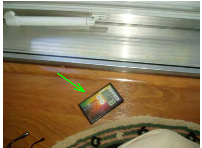
front door is noted with low moisture content...good...threshold and weather stripping is good...at door....
