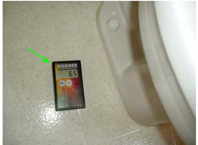
no high moisture is noted at toilet at floor....good..
