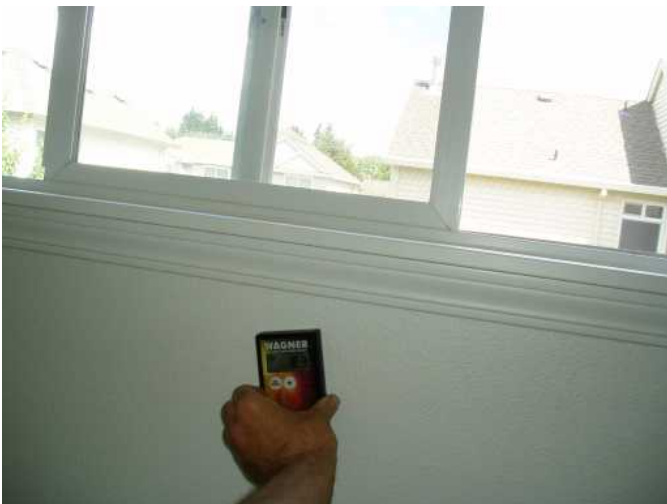
master closet window worked fine...did moisture check of walls around windows and at random, 5.5% - 7.7% good...
