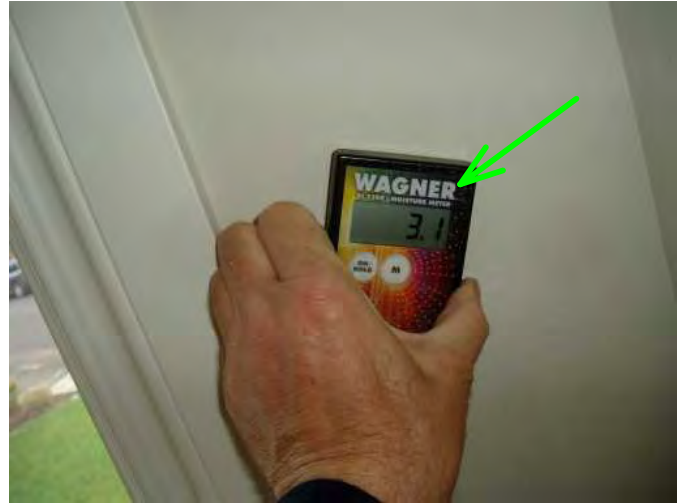
check all exteriors walls around windows and doors and noted moisture is low...very good...20% or higher is issue...
